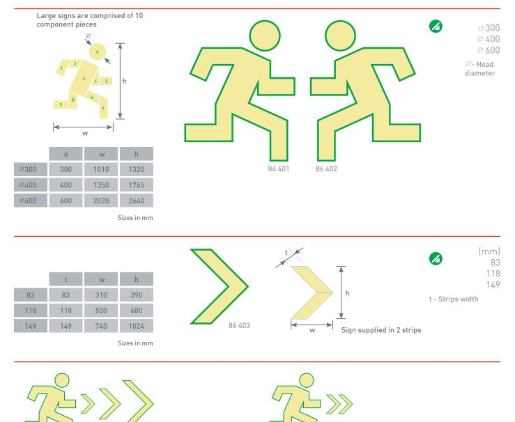
Large signs can also be used in conjunction with arrows of increasing size to emphasise the direction of the emergency escape route and exists. Dependent on the size of the large sign installed, it is recommended that the accompanying arrows should be proportionately sized. For example, a symbol with the head diameter of 300mm should have an accompanying arrow 83mm wide.
